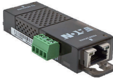
Figure 5-3: Second-generation Environmental Monitoring Probe
