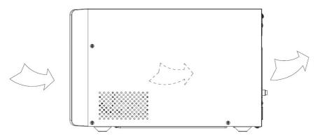
**■** Figure The Air Flow Diagram
