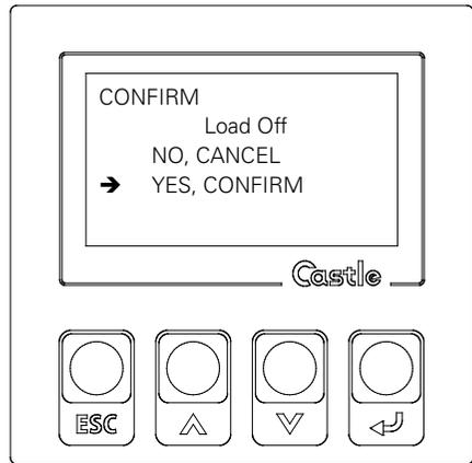
The 3C3 PRO series can start and operate with battery in the absence of AC mains supply, with a panel display similar to that in the case of AC supply. You can just follow the instructions displayed on the panel to start or shut down the UPS with battery:
