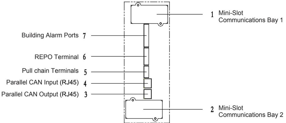
1 (2). Expansion slots: Slots exclusively available on the 20KS-200KS models and only accessible by users with special requirements. Standard users have no access to the slots.
