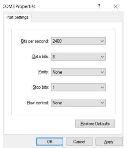
Enter the "PI" or "Q1" command and press Enter to see if there is a reply from the UPS. If the serial port cannot be opened and shows that it is occupied, you need to close the software occupying the serial port or use another serial port. If the UPS does not reply, you need to check whether the serial port cable is loose or whether the UPS/computer serial port is normal.
