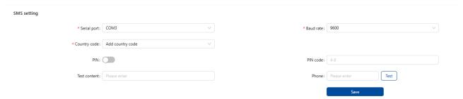
Serial port: The serial port connected to the SMS Modem
