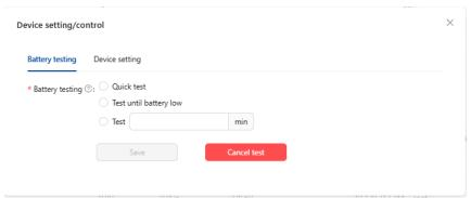
Set UPS parameters (different UPS supports different parameters)
